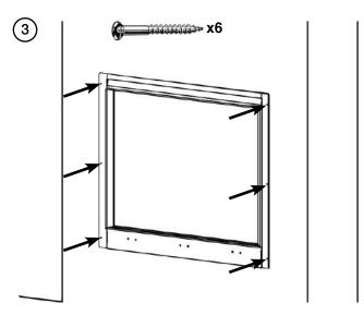
Fit non-combustible board to the chimney breast around the appliance, using the distance to combustibles detailed
