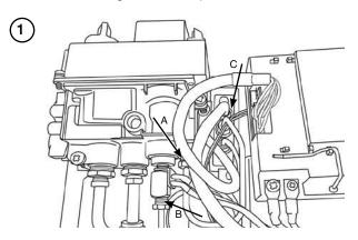
The pilot bracket can now be withdrawn from its cradle.
