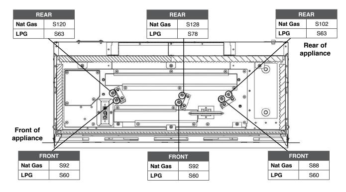
NOTE: Aeration Holes are in each leg of the burners. These holes are different sizes at the Front and Back for each individual leg.
