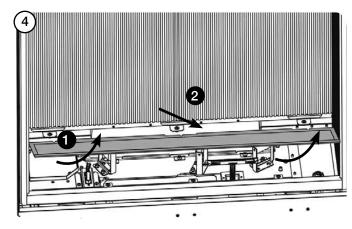
WHEN REPLACING THE MESH TRAY TAKE CARE NOT TO DAMAGE THE LOG BURNER BRACKETS, PILOT AND CROSS LIGHTER. REPLACE THE FRONT SCREWS FIRST BEFORE TIGHTENING THE REAR SCREWS.
