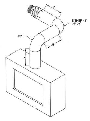
When A = 1.0 to 1.499 metres B + C = 1.0 metres maximum When A = 1.499 metres to 3.0 metres B + C = 4.0 metres maximum
