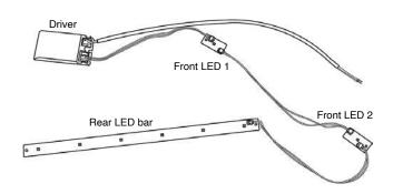
THE LED'S ARE FRAGILE. HANDLE WITH CARE. ONLY HOLD THE LED BOARDS BY THE EDGES TO AVOID CONTACT WITH THE TOP OF THE LED'S.
