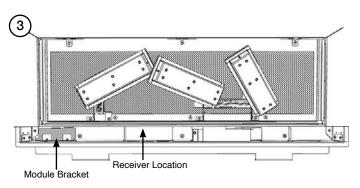
The receiver is located beneath the Main Control Assembly, close to the pilot area.
