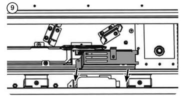
Disconnect the LED lead and the Receiver lead from the power module, if fitted, disconnect the Wi-Fi lead from the Wi-Fi module (if installed.
