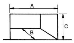
NOTE: If using natural materials for the back panel of the fireplace, it is recommended that it is constructed from three or more sections to prevent cracking. Resin based materials may not be suitable. This appliance is an effective heat producer and attention must be paid to the construction and finish of the fireplace.
