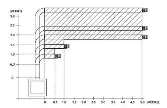
Start of bend to centre line of horizontal flue 170mm. Centre line of vertical flue to end of bend 220mm.
