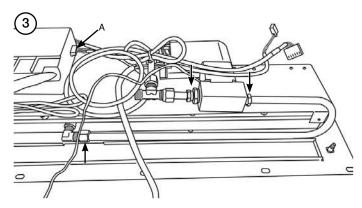
Remove the Solenoid plug from the Control Box (A).
