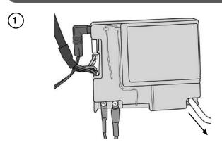
Carefully cut cable ties from the vidaflex and disconnect the lead from the electrode.
