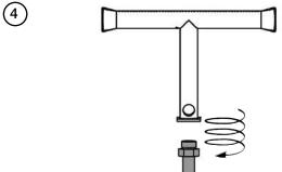
Replace with the correct size Injector and refit all components in the reverse order.
