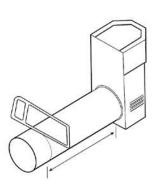
Terminal dimensions: 395 x 200 x 200 mm (H x W x D) Guard supplied Cut to length as required on site.
