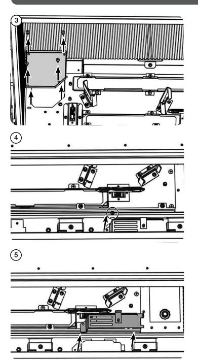
Disconnect the Mains Lead Plug, the LED leads and the receiver lead from the Module and the Wi-Fi box (if installed). **DO NOT REMOVE THE WIRES FROM THE PLUG.**
