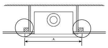
This diagram shows the minimum clearance position when installing the appliance into studwork - it is vital to ensure the opening is wide enough to accommodate the fixings for the front.
