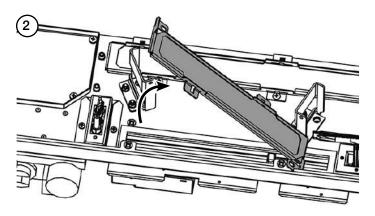
Remove the 2 screws holding the LED boards to the Control Assembly by inserting a screwdriver through the gap previously covered by the glass bracket.
