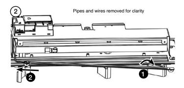
Undo the three nuts shown and free the solenoid from the pipework.
