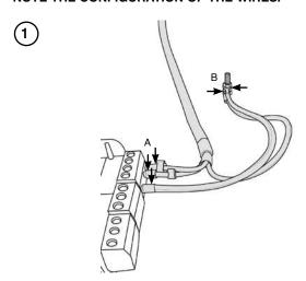
Remove the nuts from the Earth stud and remove the two Ring Terminals (B).
